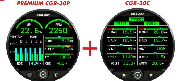
**Specifications:** Each instrument fits standard 3 1/8" Hole. Dimensions: 3.125" x 3.125" x 4.45" depth. Accuracy: 1/2%. Viewable in direct and indirect sunlight. **FAA approved, STC'd and TSO'd as Primary Replacements.**
