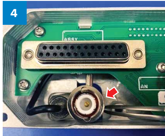
Reposition COM coax inside retrofit adapter to prevent interference with KX 200.
