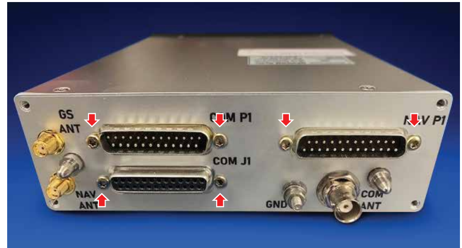
M3x5 screws installed.
