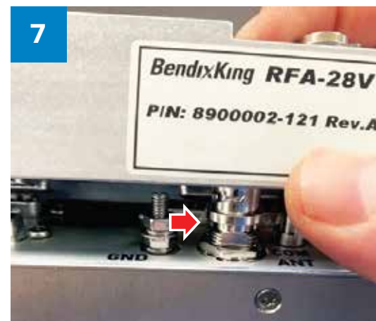
Connect and lock the COM antenna connector to the connector on the KX 200.
