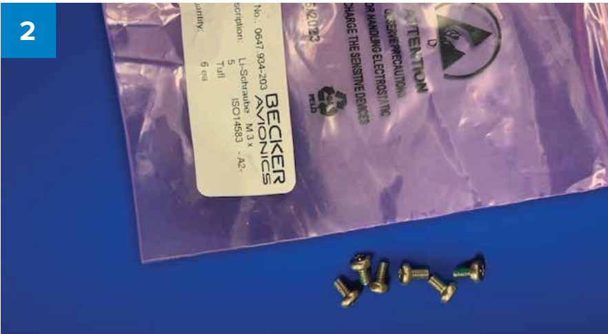
Install (6) supplied M3x5 screws using an M4.5 hex socket wrench. Torque screws to 9 in/lb.
