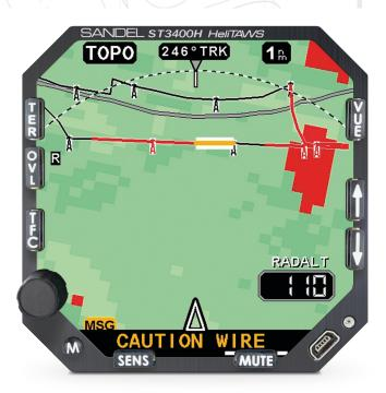
Sandel ST3400H HeliTAWS<sup>°</sup> is the industry's first multihazard avoidance system for helicopters that alerts against wires, terrain, and obstacles, utilizing WireWatch<sup>°</sup>— advance defense against wire strikes. It further enhances the operational awareness in the cockpit by helping helicopter pilots avoid transmission lines whether they are powered on or off.
