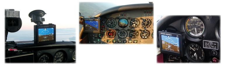
The D1 Pocket Panel is a true artificial horizon based on the same technology that drives Dynon's Electronic Flight Instrument Systems (EFIS).
