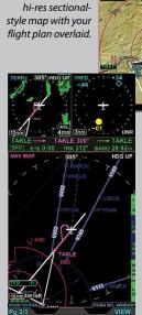
Three dedicated displays in one; with your choice of content in each. Shown here: monitor potential traffic and terrain hazards, while tracking progress along your flight plan on an IFR view optimized for night flight.
