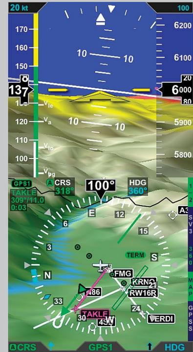
Evolution Synthetic Vision is an optional expansion to the Evolution 1000 Pro PFD that presents a real-time 3D rendered view of terrain, traffic, and other hazards. The synthetic rendering simulates the view from the cockpit on a bright day, so it's especially helpful to provide situational awareness when flying during conditions of reduced visibility or darkness.
