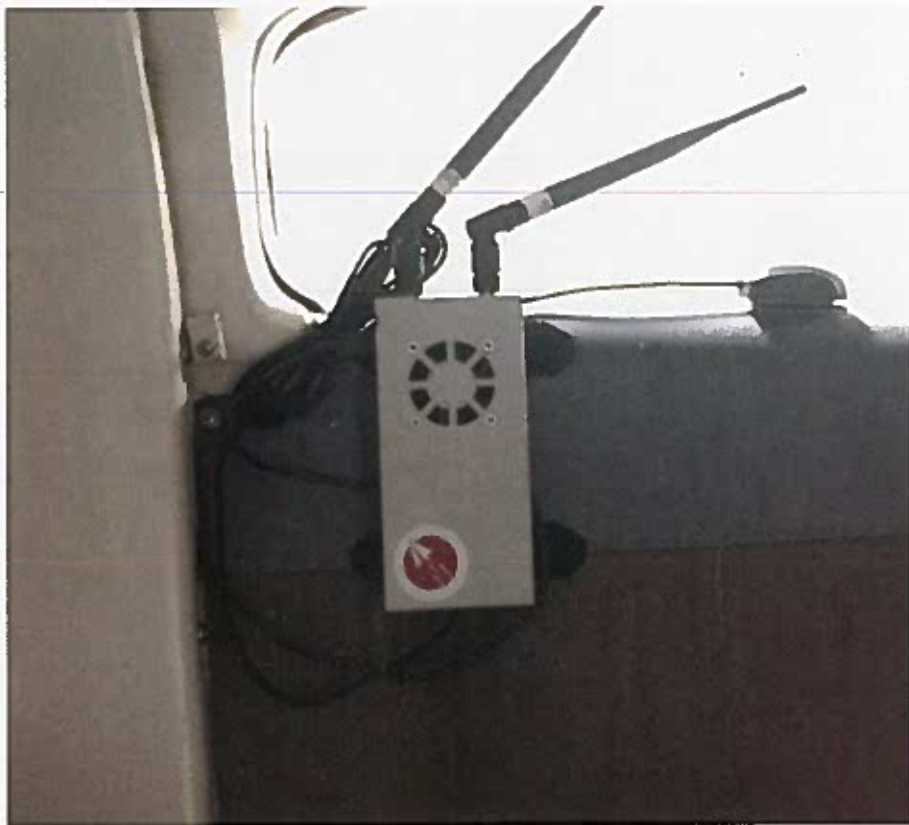
The Open Flight Solutions' "FlightBox" Velcro-mounted to the baggage compartment sidewall. Note the two antennas and the WAAS GPS.
