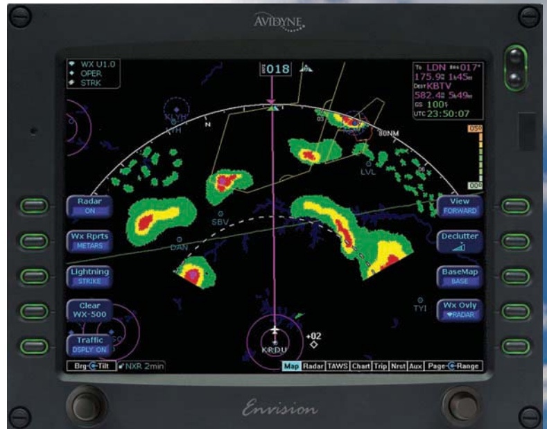
The FlightMax EX5000 interfaces with several digital radar models, which can be overlaid right on the map page or viewed on a dedicated radar page.
