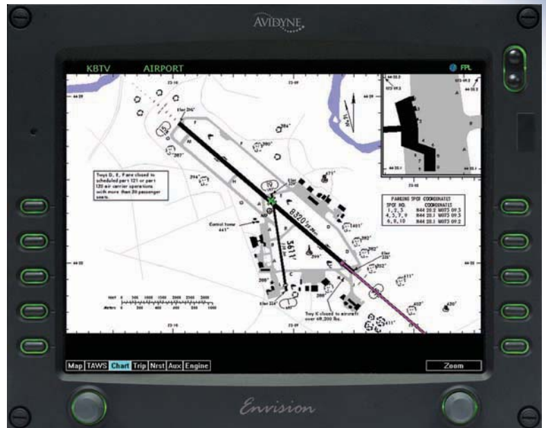
CMax automatically switches to the destination airport diagram when ground speed drops below 40kts and shows your aircraft's position on the runway or taxiway.
