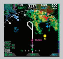
Evolution Hazard Awareness (EHA) presents an integrated display of potential flight hazards directly in front of the pilot. EHA is a standard, built-in feature of the Evolution MFDs and is an optional software upgrade on the Pro PFD. EHA enables the display of traffic, datalink weather, and WX500 Stormscope® data from compatible sensor systems.
