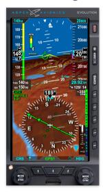
Aspen's innovative Evolution Angle of Attack (AOA) indicator provides the pilot a visual display of the AOA trend and the approximate available lift simultaneously in all phases of flight.
