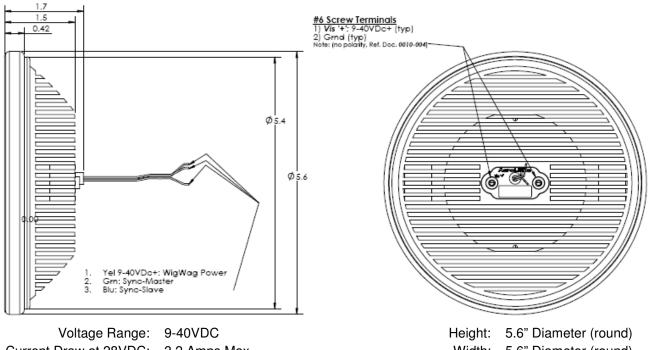
Voltage Range: 9-40VI Current Draw at 28VDC: 3.2 An Power Consumption: 90 Wa Pulse Light Feature: Built Ir Wig Wag Sync: Built Ir Thermal Protection: Built Ir Landing Lens Candela: 120,00 Landing Beam Angle: 10 Deg Total LED Lumens: 5000+ LED Count: 9
