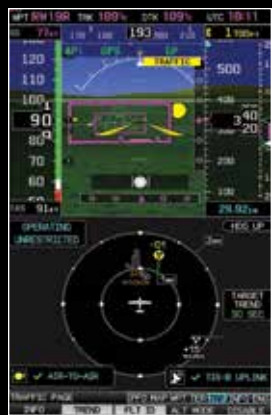
ADS-B input 1 enables subscription-free weather and advanced traffic features like TargetTrend™ relative motion.
