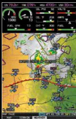
Optional XM WX™ satellite weather can overlay on the G3X moving map 2
