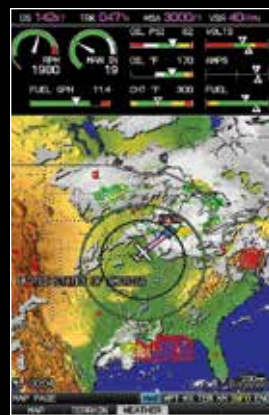
How far can you go? Graphical range rings are based on real-time fuel flow calculations
