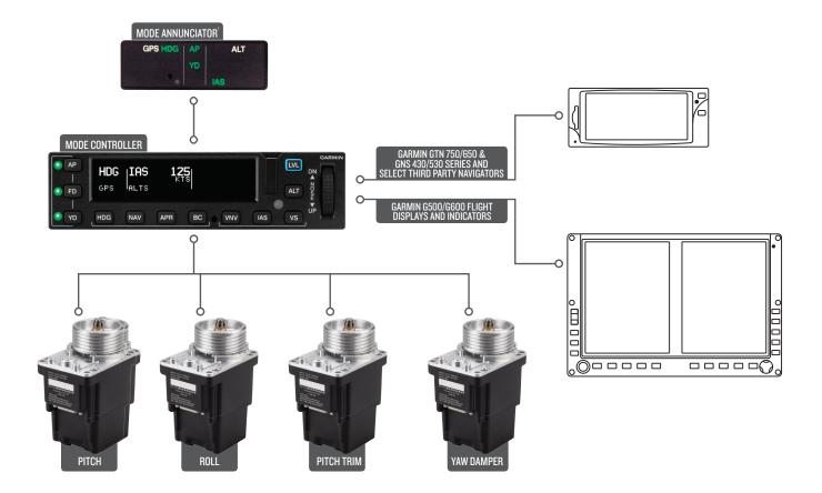
In addition to traditional autopilot capabilities such as altitude hold, vertical speed and heading modes, the GFC\* 600 also includes:
